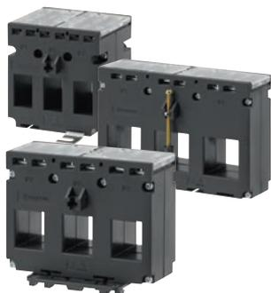
A range of 3-in-1 current transformers combine three traditional current transformers in one moulded case. 3-in-1 current transformers can be directly installed next to a three-phase moulded case circuit breaker, thus saving installation time where fitting three standard individual current transformers would be required. The M3N1 range of current transformers offers primary currents between 60-630A with 5A secondaries with up to Class 0.5 accuracy performance.
