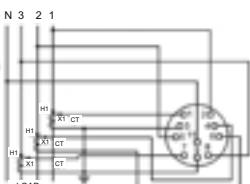
Fig. B2 Models 078-218 Wattmeter 3-phase 3-wire unbalanced load
