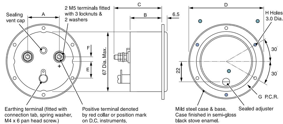
\*When fitted with terminal shunt for ranges above 20 amps.
