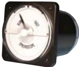
The Crompton Instruments AC synchroscope measures and displays the frequency difference of two power sources. Monitoring the display allows the user to connect two synchronised AC power systems together. This can help prevent the potential damage caused by connecting two unsynchronised power sources.
