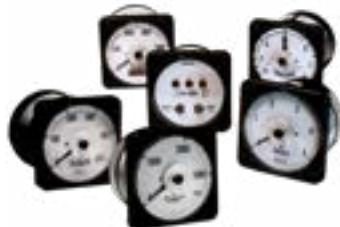
High quality range of switchboard instruments with Class 1 accuracy and which complies with American ANSI-C39.1 (1981) specifications. Available in 4 1/2" case size, the rugged design characteristics meet the needs of the most demanding environmental applications. This extensive range of analogue and digital/analogue meters utilises high shock and provides 1% accuracy for all RMS AC and DC ranges. The range offers various customised options and features.
