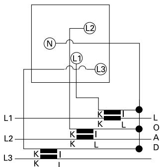
AC voltmeters 3-phase 3-wire
