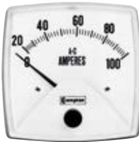
A robust range of short-scale 3½" surface mount panel meters offering IP55 protection and featuring a wide view contoured window. The Fiesta range includes iron vane and moving coil AC and DC ammeters and voltmeters, elapsed time and frequency meters and is ideally suited for demanding environments. Options include panel gasket.
