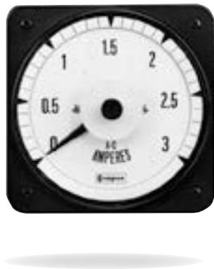
This range of self contained, pivot and jewel moving iron meters feature 250° linear scale. AC instruments are available with true RMS converting circuit or RMS compensated rectifier. While types of frequency meters can be damaged by transient supply voltage spike, Crompton Instruments 007-41 frequency meters can withstand, without damage, 10 successive transient spikes of 1250 volts. The range offers c-UL-us certification.
