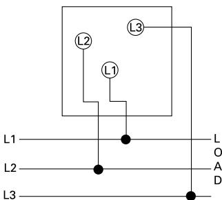
AC voltmeters 3-phase 4-wire
