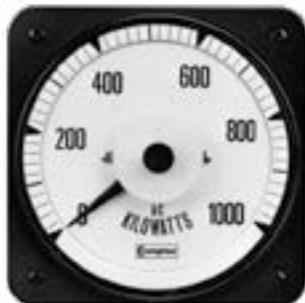
The Crompton Instruments Switchboard series of AC Wattmeters and VArmeters incorporate a DC moving coil, pivot and jewel indicator with a micro-circuit watt transducer PCB to read power on single or three phase systems with optional transformer isolation. The most frequently selected wattmeter scale marking for common current and voltage transformers are listed on the following pages. In addition, these instruments may be supplied with zero-left or centre-zero scale.
